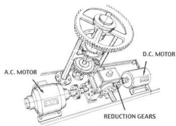
ELECTRIC LENS TURNING MECHANISM
