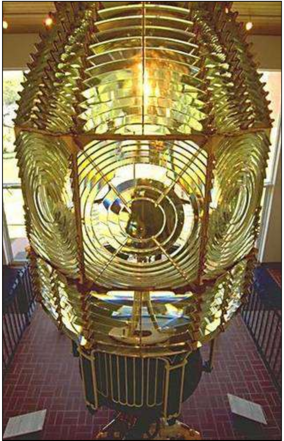
Planier Light-Fresnel 16 first order, 16 section lens
